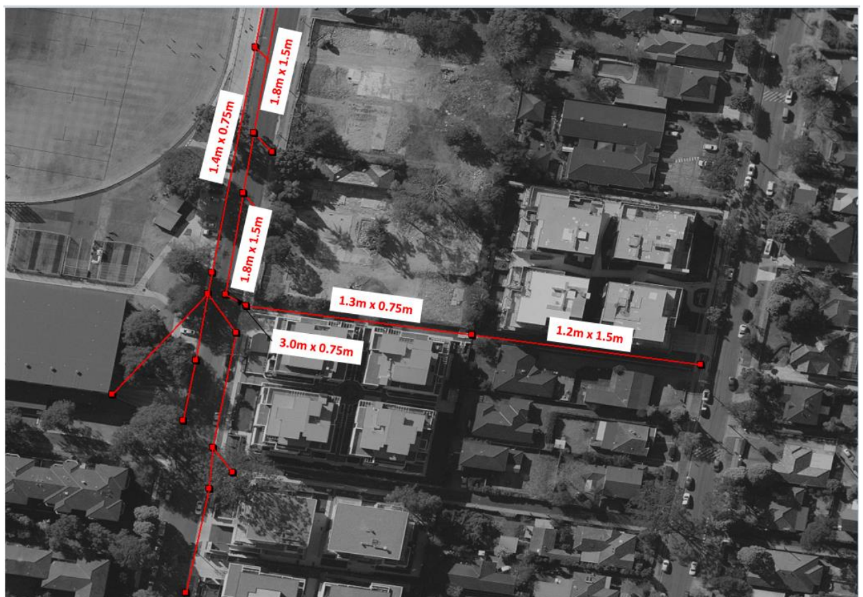
Image 2: Existing Stormwater network
