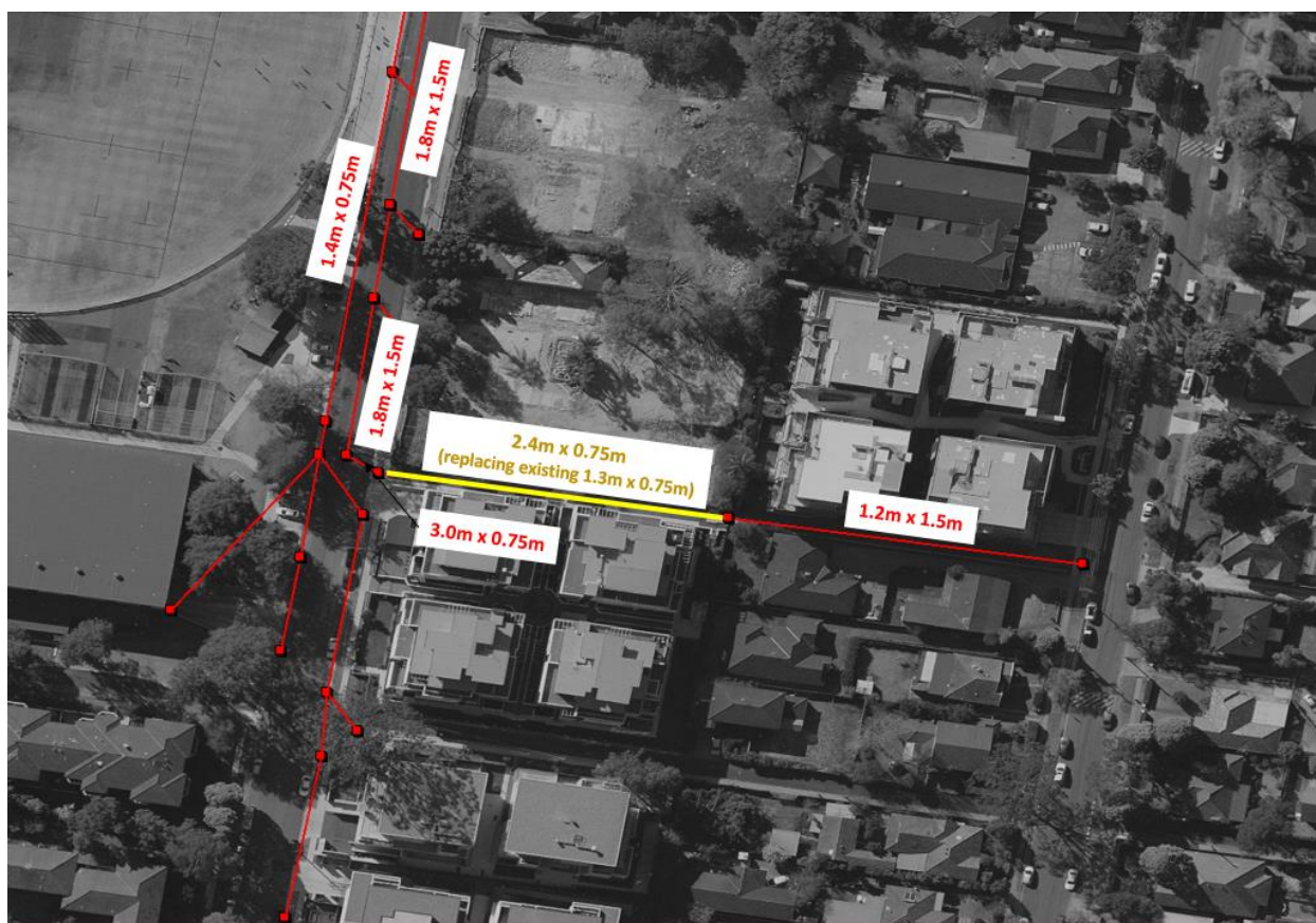
Image 5: Proposed Culvert Upgrade
